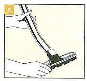
CONNECTING WAND TO FLOOR AND WALL BRUSH: Insert the end of the curved metal wand into the floor and wall brush. Align the button lock on the wand with the guide on the brush collar. Slide the button into the guide to engage the lock.
