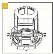
The Rainbow power cord attaches to the back of the power unit. Sliding holders and a stationary holder on the exhaust vent panel door are used to store the power cord. To use the power cord, simply retract the cord caddy holders using the finger grips (see illustration), and cord is then accessible.
