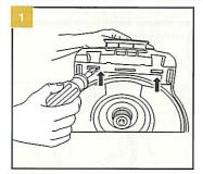
Using a screwdriver, remove the panel from the back of the machine by pressing up on the two latches on the underside of the rear panel. Move the bottom of the rear panel towards you, lifting up.
