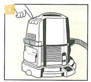
Connect electrical cord to wall outlet. Toggle the speed" setting (>>). Use this control sleeve for full power. setting for normal cleaning operations. To turn the Rainbow off, toggle switch to "OFF" position (O).
